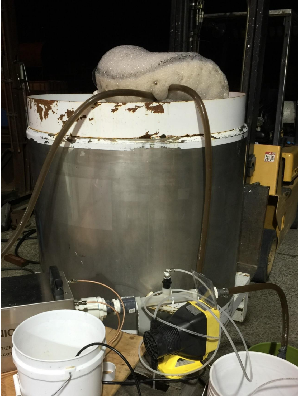
AOP Processing of RCRA Subtitle D Landfill Leachate without AMEOX™ Treatment for Foam (and PFAS) Management
